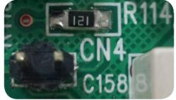
Taking the GMV5 DC inverter system for example, as shown in the figure above, there are two pins located at CN4. The jumper-shorted two pins are equivalent to a matched resistance.
