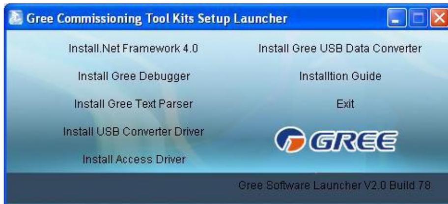
For the first time to use Gree Commissioning Tool Kits, install these programmes: .Net Framework 4.0, USB Data Converter, Access Driver (necessary for versions below OFFICE 2007), Gree Debugger.
